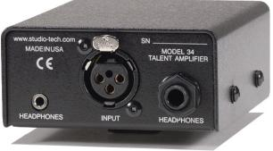
The Model 34 is compatible with virtually every standard broadcast IFB and party-line intercom circuit. This type of circuit typically uses 3-pin XLR-type connectors for interfacing with connected equipment. XLR pin 1 serves as common for DC power and audio. Pin 2 provides DC power and, in the case of a dual-channel circuit, DC power and channel 1 audio. Pin 3 provides channel 2 audio in dual-channel systems or channel 1 audio in single-channel systems.
